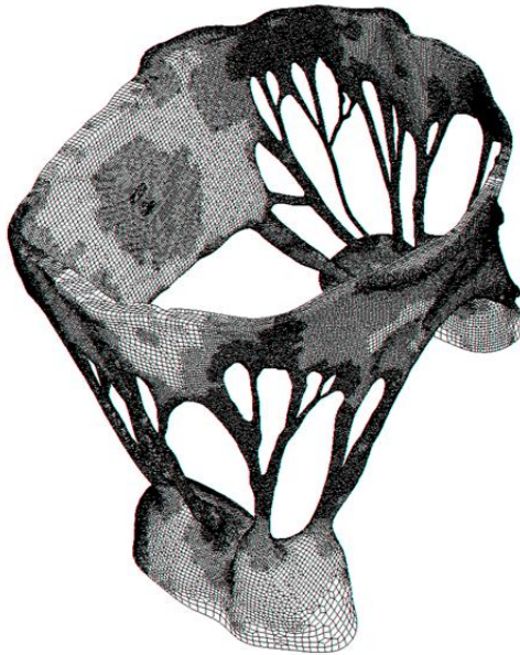
Figure 8-29 Highly resolved mesh of the anatomically accurate mitral valve model generated from micro-computed tomography.
