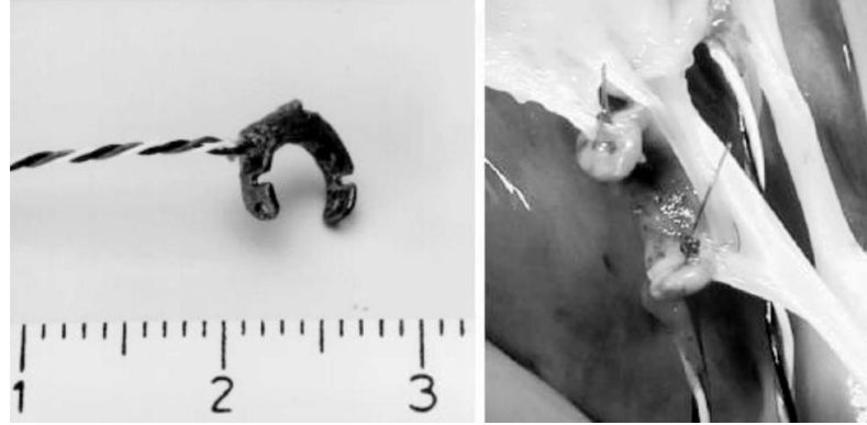
Figure 2-8 Miniature C-arm force transducers selectively record chordal forces throughout the cardiac cycle (Image adapted with permission from Nielsen et al. [8]).
